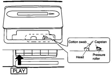
The head assembly, capstan and pressure roller are in constant contact with the tape. If these parts are dirty, the sound quality will be impaired. Periodically, clean these parts as shown.
