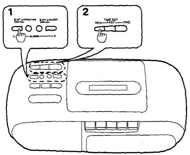
1 Press and hold the alarm 1 (or 2) display/adjust button.
